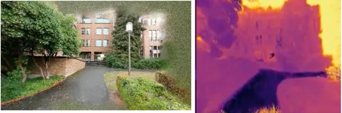
Figure 7. BayesRays uncertainty estimation. Left: NeRF-rendered frames along the spline trajectory. Right: corresponding uncertainty map ( \delta field). Yellow = highest uncertainty (sky and far-field foliage, poorly constrained by training views); dark teal/blue = lowest uncertainty (ground-level geometry and building facades) (video available at https://github.com/Leopardise/FLASH/blob/main/Uncertainty_analysis.mp4 ).
